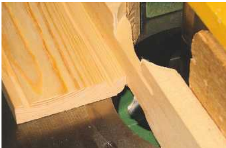
▲ Pic.4 You'll need to cut an ovolo mould on the outer facings as shown
